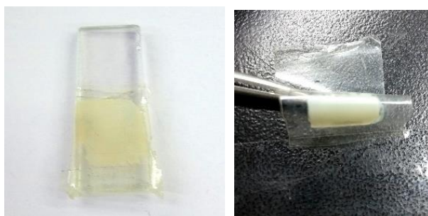
S6. Working electrode: Membrane supported in ITO glass.
